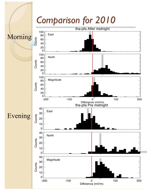
Histogram of differences (**THApfa**) for two groups of data during 2010. These differences are plotted for the x-(east), y-(north), and the magnitude components.
