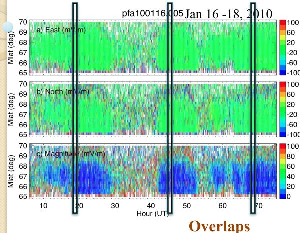
E-perp measurements by the ISR at Poker Flat during Jan 16-18, 2010. a) East component, b) North component, c) Magnitude. (Data are from http:// www.openmadrigal.org)
