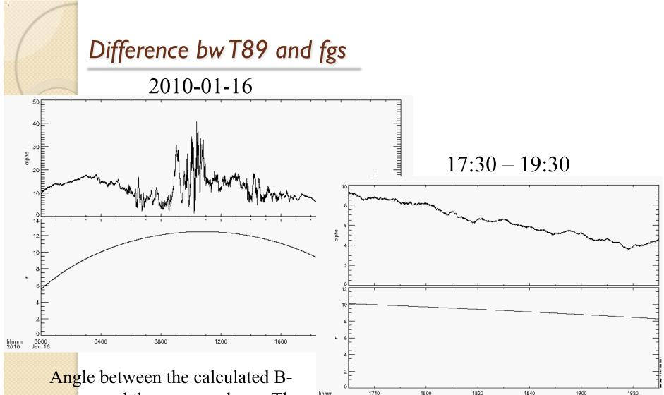
vector and the measured one. The distance of the spacecraft to the Earth's center is plotted at the bottom panel.
