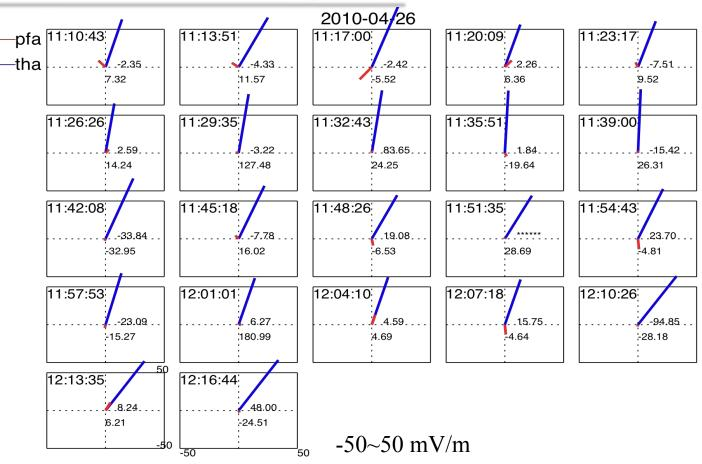
E-x (east) and E-y (north) for THEMIS (blue) and ISR (red) for each 3min overlap on Apr 26, 2010. The plotting range is 50 mV/m for both directions.
