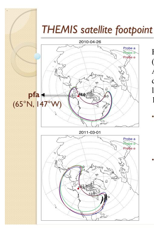
Footpoints of the THEMIS satellites (a, d, e) for one day. The top plot is for Apr 26, 2010. The bottom one is for a different day. The red dot gives the location of the ISR at Poker Flat (65°N, 147°W).
