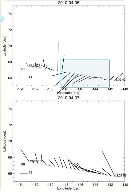
Difference vector between Tha and ISR for each overlap on one day. The vector is scaled in x- and ydirections.
